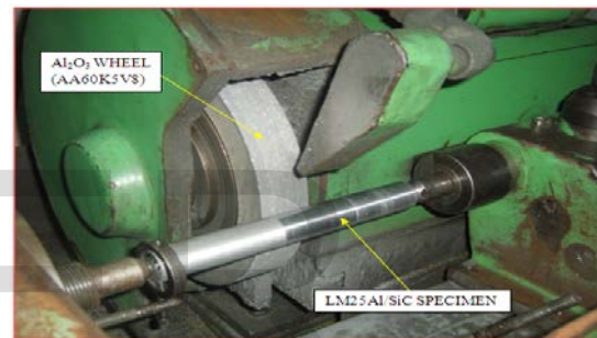
FIGURE 4 CYLINDRICAL GRINDING SET-UP
